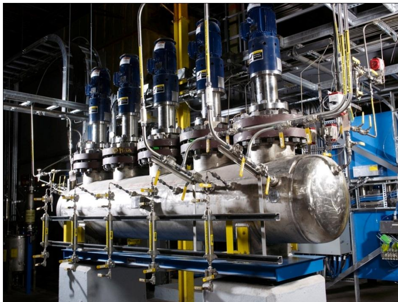
Figure 4 - CESL Gold Demonstration Plant Pressure Cyanidation Vessel
