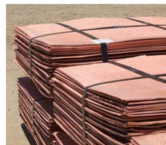
LME Grade-A copper cathodes
